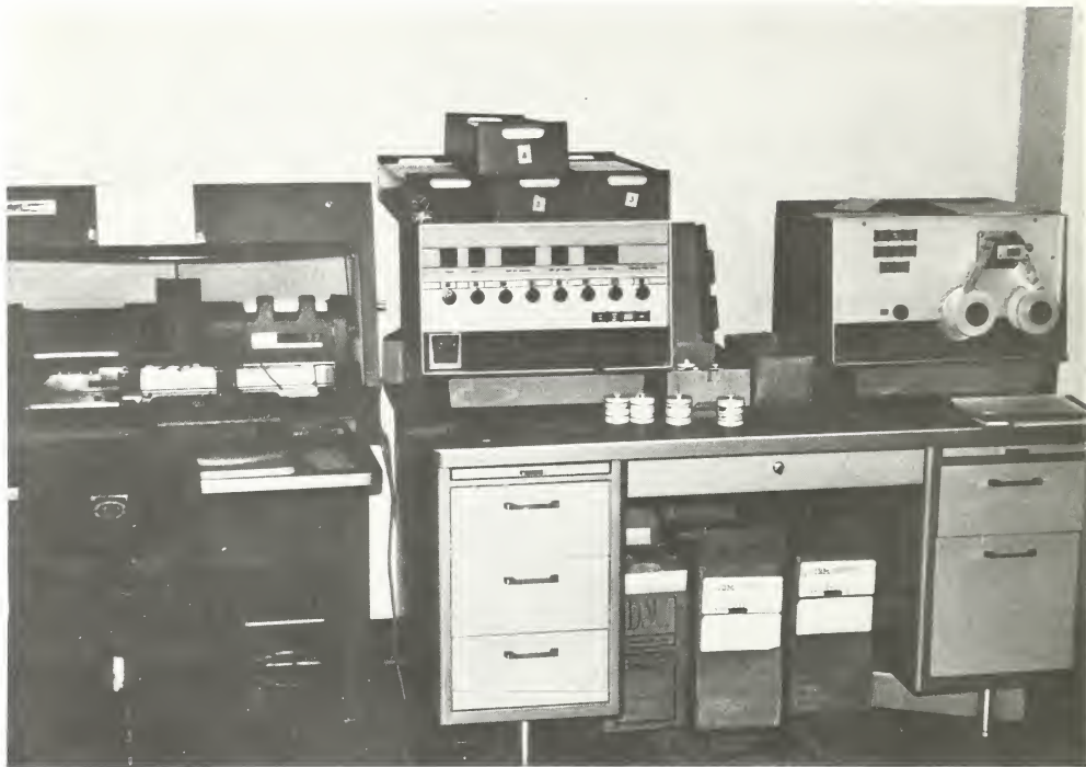
FIGURE 10.—By means of the converter unit (center) the tidal data already punched on tape (right) are transferred onto punched cards (left) which are then fed into an electronic computer for printout, tabulation, and subsequent analysis.
